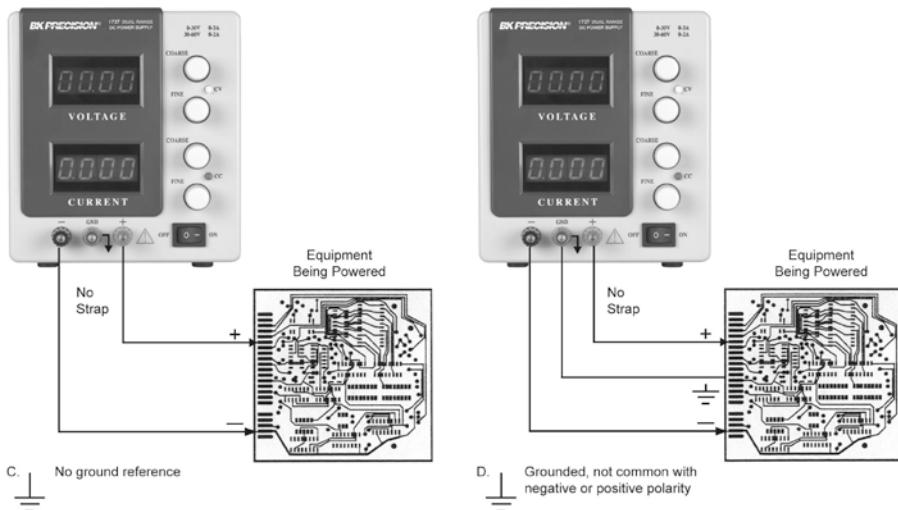
**Figure 3 (C and D) - Grounding Possibilities**
