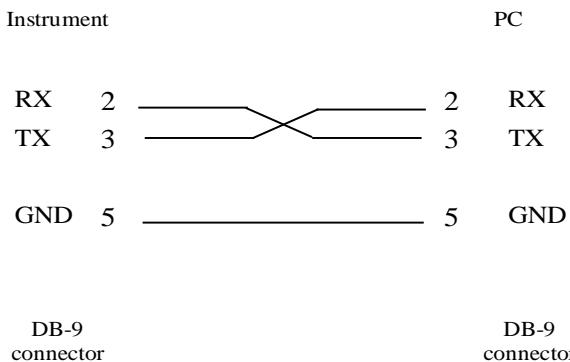
**Figure 10 - RS232 Cable Pin Diagram**
