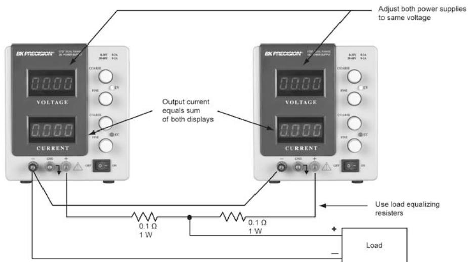
Figure 9 - Connecting Two Power Supplies in Parallel
