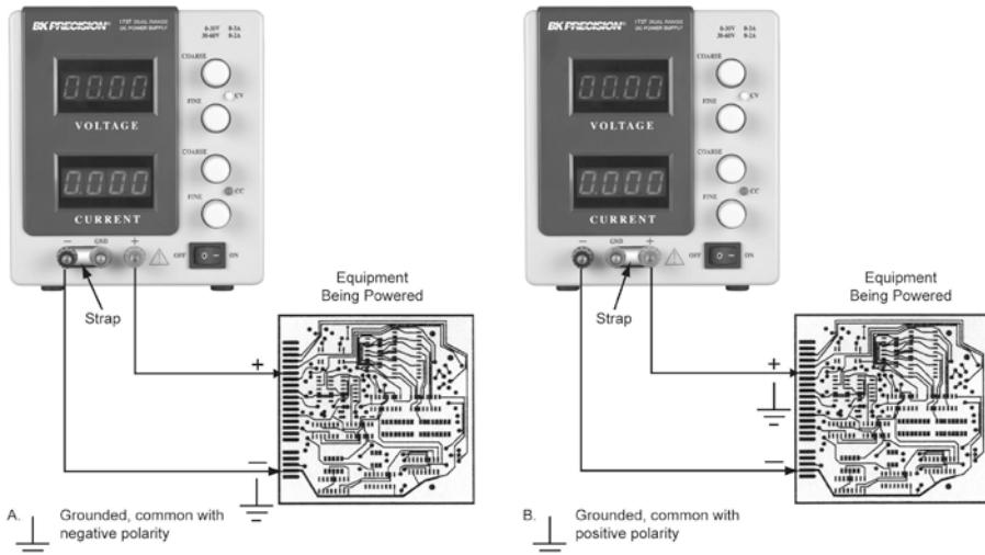
**Figure 3 (A and B) - Grounding Possibilities**
